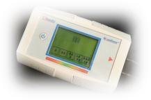
Hand held meter reads a 'drop' moisture scale from the in-dressing sensor
